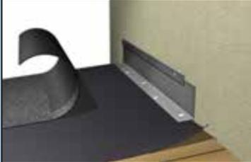
The wall flashing no. 1. is used for the production of professional roof and connections on the roof and facade. It is the connecting plate between the roof surface and the vertical component. The use of the profile ensures controlled water drainage on the roof surfaces and protects the covering from penetrating water. The universally applicable wall flashing is suitable for many roof coverings and gives the roof and facade a visual Rounding.
